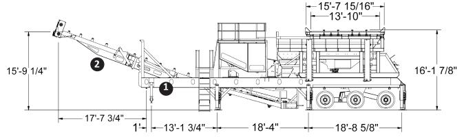
3054 Jaw Plant Less Feeder Hopper King Pin Weight: 50,400 lbs Axle Weight: 60,260 lbs Feeder Hopper King Pin Weight: 24,290 lbs Axle Weight: 34,330 lbs
