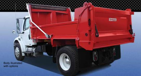
The MS-HD is designed for light to medium-duty applications (sand, gravel & light excavating). It is THE body of choice when weight is critical. The design ensures minimal weight while providing sufficient ruggedness to sustain the effort.
