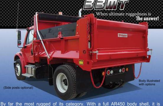
By far the most rugged of its category. With a full AR450 body shell, it is unquestionably the best suited to sustain constant abuse (heavy duty excavating, demolition). Furthermore, the AR steel provides this body with an incomparable wear-resistant factor as well as the ultimate resistance to impacts.
