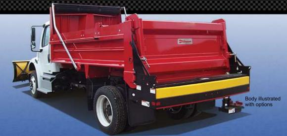
If price is your main focus, the MS1 (medium-duty) or the MS0 (light-duty) can get it done for less. Constructed of grade 50 steel with an AR200 floor center piece, both the MS1 and MS0 are up to the task.
