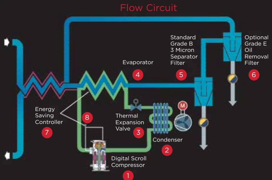
While the compressor continues to run, the Energy Saving Controller (7) automatically energizes and de-energizes the solenoid valve (8) to load and unload the compressor.
