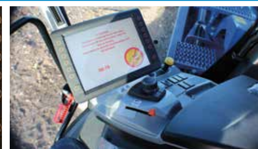
The single-joystick control, load-sensing and touchscreen display make for easy operation.
