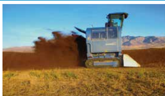
Independently controlled track clears guide material to the drum and "float" to fit any pad.
