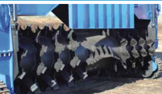
Large diameter drum maximizes homogenization and oxygenation of the windrow material.
