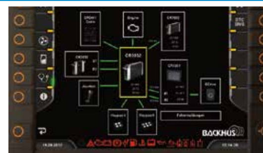
Self-diagnostic CAN bus system provides real-time feedback and alarms displayed in text format.
