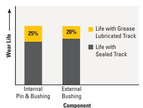
Increased wear life of pin and bushing means more sprocket and link life is utilized.
