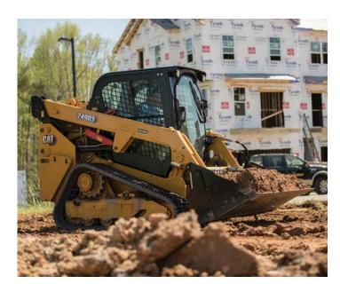
Keeping the full length of track on the ground provides the most traction and takes advantage of the machine suspension. You can get excellent results and maximize the life of your undercarriage by backdragging with loader arms, using the FLOAT function. If more down pressure is needed, the CTL suspension system will allow for additional down pressure to be applied without raising the undercarriage off of the ground. Add only the pressure required to smooth the surface.
